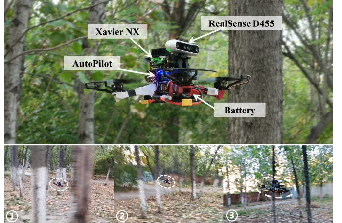
Fig. 9. The physical platform and real-world experimental scenario. ① - ③ are the snapshots of the corresponding positions in Fig. 10.
